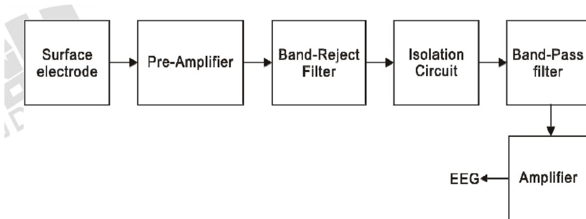
Block diagram of EEG measurement circuit.
