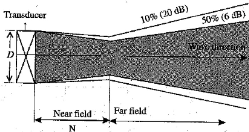
Fig. 3.29 Beam profile of a transducer
