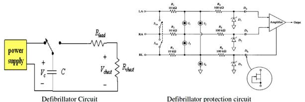
The protection circuit may be only the series resistors or the zener diodes or the neon glow lamps or the FET diodes.
